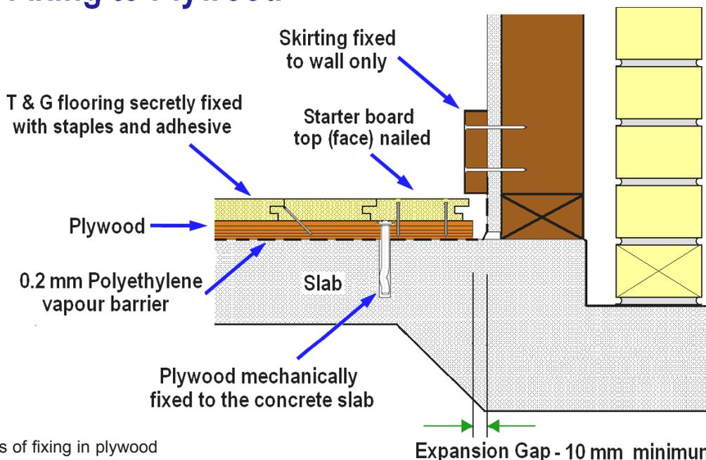
Figure 3 - Details of fixing in plywood
