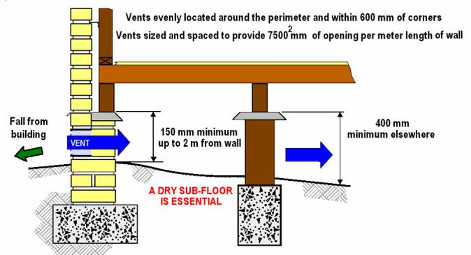
Figure 1 - Sub-floor Ventilation
