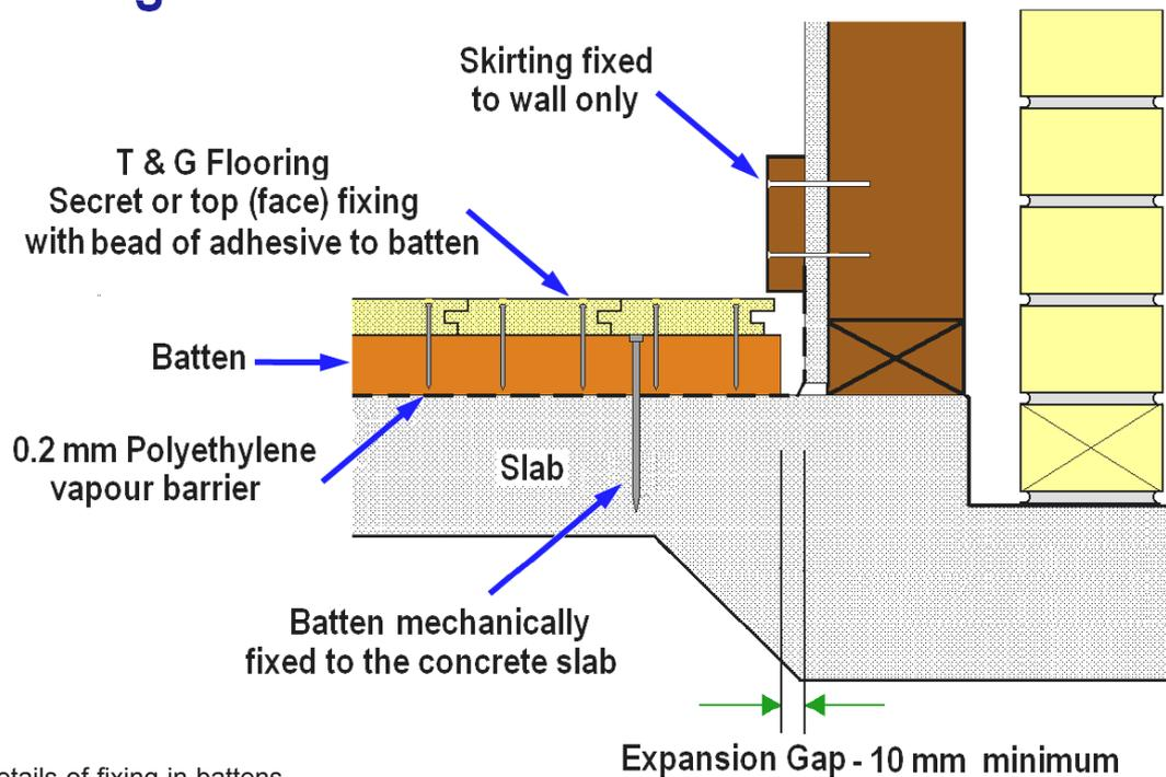
Figure 4 - Details of fixing in battens
